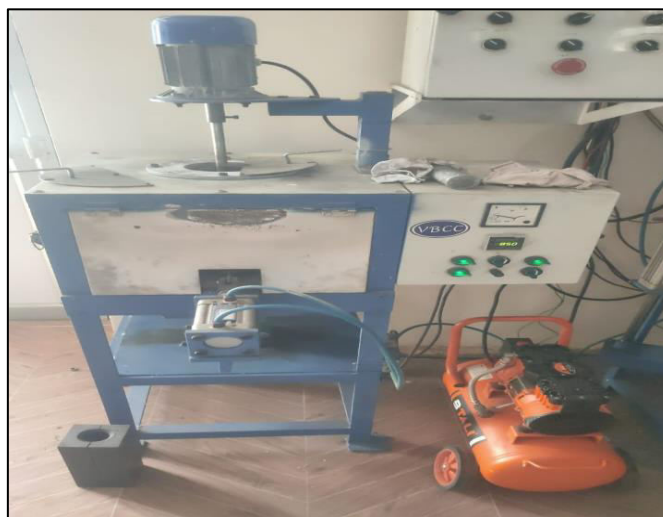
Figure 3: Stir casting setup used for synthesizing the composite
